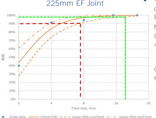
95% confident that we can detect a 7.4mm flaw with a POD of 90% Maximum brittle decohesion
