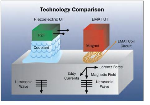
Electro-Magnetic Acoustic Testing (EMAT)
