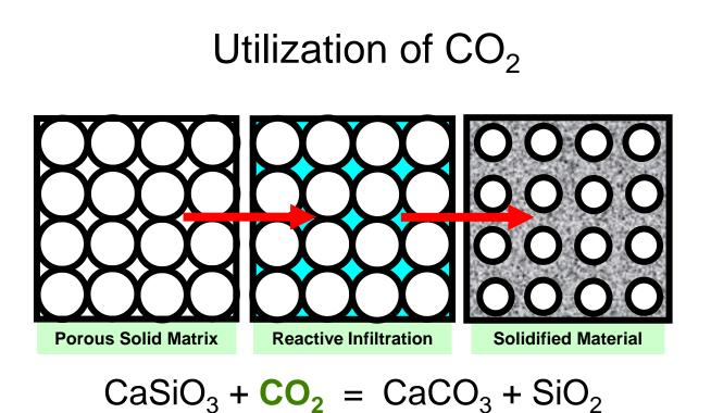
1<sup>st</sup> commercially manufactured carbonate-bonded material
