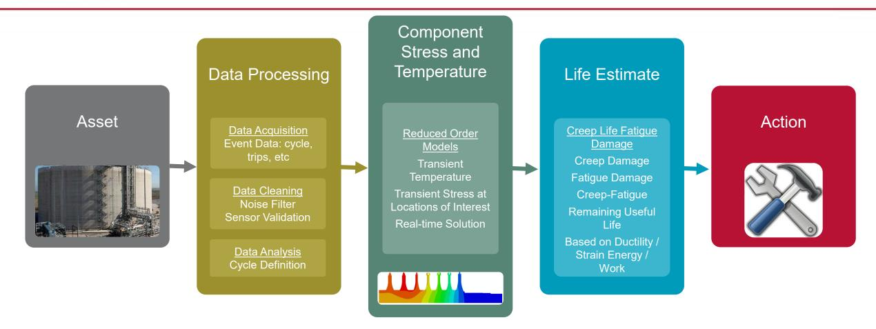
The Condition Based Maintenance approach uses data from individual assets to determine life usage to inform and tailor maintenance actions
