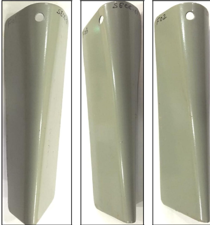
Figure .2 Photographs of the Flexibility Tested Samples
